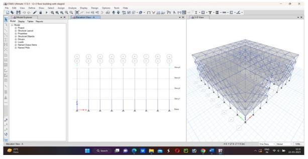
Figure 1: Elevation and 3D View of G+3 Diagrid Building
