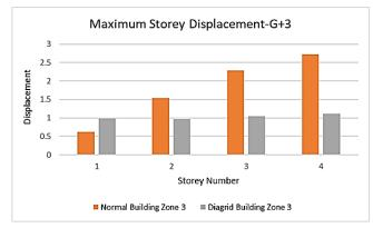
Figure 8: Graphical representation of maximum storey displacement in Zone III
