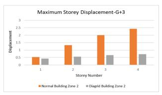
Figure 7: Graphical representation of maximum storey displacement in Zone II
