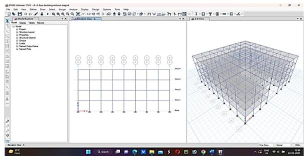
Figure 2: Elevation and 3D view of G+3 Conventional Building
