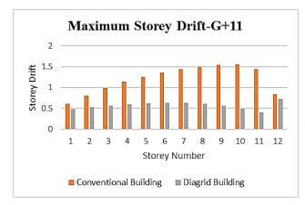
Figure 9: Graphical representation of maximum storey drift in Zone II
