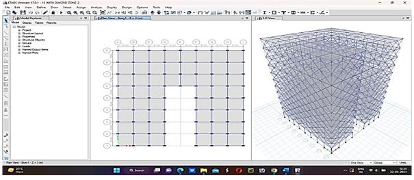
Figure 4: Plan and 3D view of G+11 Diagrid Building
