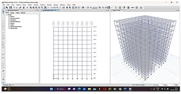
Figure 3: Elevation and 3D view of G+11 Conventional Building
