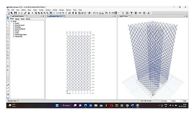
Figure 6: Elevation and 3D view of G+19 Diagrid Building
